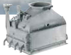
Air Cooler for an Air-Cooling- Unit (AOA Apparatebau Gauting) for food cooling used in the Airbus A380
