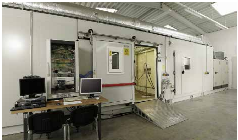
Wind tunnel for performance measurement of large cooling systems
